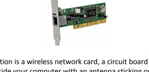
Another option is a wireless network card, a circuit board that is installed inside your computer with an antenna sticking out the back. This type of NIC requires a wireless transmitter, which we will discuss in a moment.
