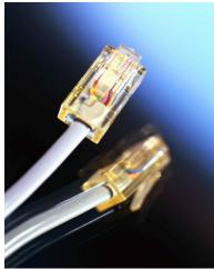
While two computers can use a special cable (cross-over cable) to physically connect to each other (NIC-to-NIC), a normal Ethernet cable (straight cable) is used in all other networking scenarios. When connecting more than two computers, you will need to use an intermediary device like a router, switch, or hub (explained below). Networking cables can come in many different kinds and lengths. For home networking a simple CAT5 Ethernet cable will be fine. This cable is usually blue or grey.
