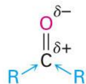
Ketone (more stabilization of \delta+ , less reactive)
